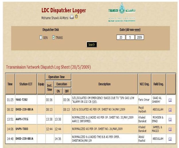
Fig.12. The electronic logging console of the DAS system.
